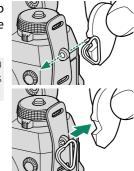
5 Pass the clip through the eyelet. Rotate the clip fully through the eyelet until it clicks closed.
