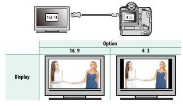
Select 16:9 to display the image so that it fills the screen with its top and bottom cropped out, 4:3 to display the entire image with black bands at either side.
