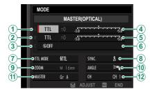
The master and remote units can be placed in up to three groups (A, B, and C) and flash mode and flash level adjusted separately for each group. Four channels are available for communication between the units; separate channels can be used for different flash systems or to prevent interference when multiple systems are operating in close proximity.
