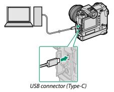
The USB cable must be no more than 1.5 m (4.9 ft.) long and be suitable for data transfer.
