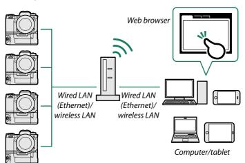
Before recording movies remotely, you will need to create a connection setting profile for use when connecting the camera to a computer or tablet via wireless or wired LAN.
