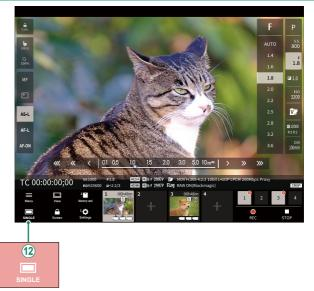
A 4-screen display button has been added. If this button is pressed, the screen display is divided into four parts to check the live views of multiple cameras at the same time.
