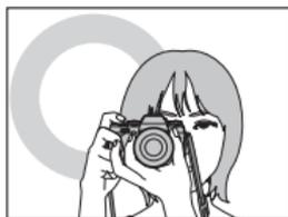
To prevent pictures that are out of focus or too dark (underexposed), keep your fingers and other objects away from the lens and AF-assist illuminator.
