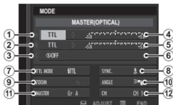
The master and remote units can be placed in up to three groups (A, B, and C) and flash mode and flash level adjusted separately for each group. Four channels are available for communication between
