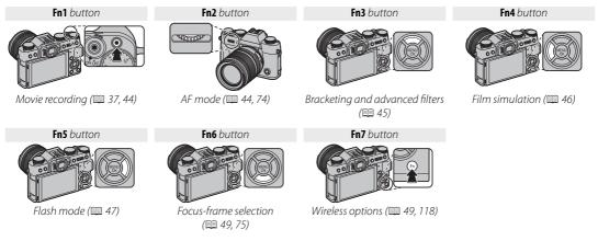
• You can also display options for any of the function buttons by pressing and holding the button.
