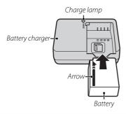
The camera uses an NP-W126 rechargeable battery.
