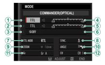
Fujifilm optical wireless remote flash control offers a choice of four channels (Channels 1 through 4) for the exchange of optical signals between the commander and remote flash units. Separate channels can be used for different flash systems or to prevent interference when multiple systems are operating in close proximity.
