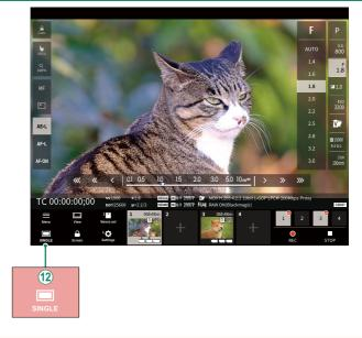
(12) A 4-screen display button has been added. If this button is pressed, the screen display is divided into four parts to check the live views of multiple cameras at the same time.
