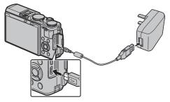
$\ensuremath{\mathbbm D}$  Be sure the connectors are in the correct orientation and then insert them fully.
