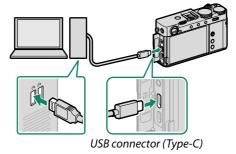
The USB cable must be no more than 1 m (3.3 ft.) long and be suitable for data transfer.
