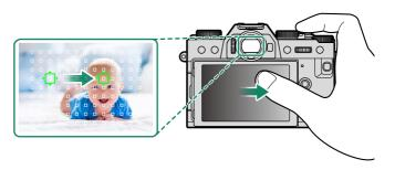
If ■ FACE SELECT ※ Is enabled when FACE DETECTION ON is selected for M AF/MF SETTING > FACE/EYE DETECTION SETTING, the face used for focus can be chosen via touch controls.
