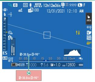
(54) If a T/S lens is attached, the shift and rotate amounts are displayed.
