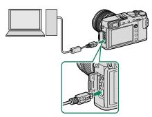
The USB cable must be no more than 1.5 m (4.9 ft.) long and be suitable for data transfer.
